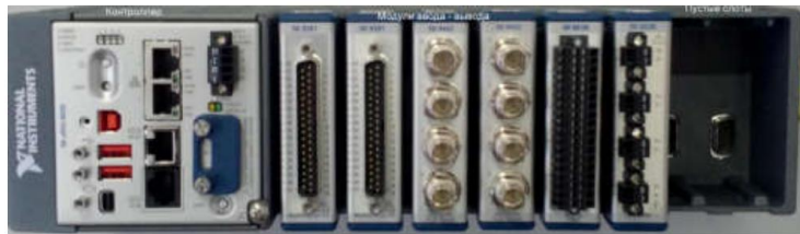
Figure 3 – cRIO-9035 controller with chassis modules
