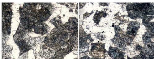
Figure 1 – Microstructure of 20GL steel before quenching
